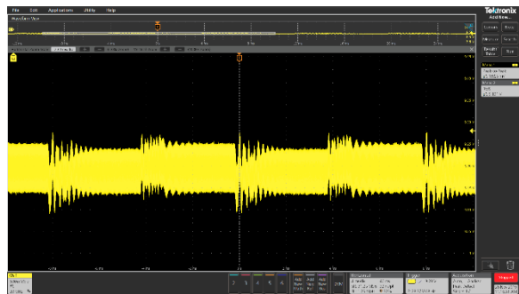
Figure 25. Transient Load on 9 V BUS
