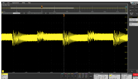
Figure 24. Transient Load on 5 V BUS
