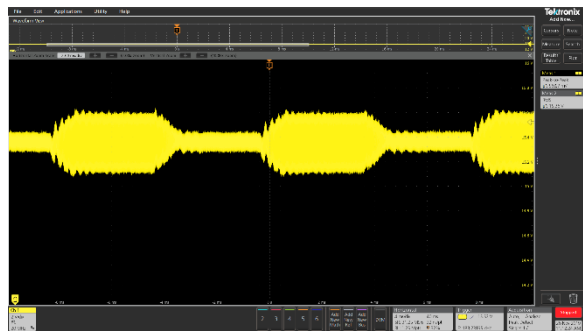
Figure 27. Transient Load on 15 V BUS
