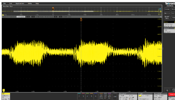
Figure 26. Transient Load on 12 V BUS
