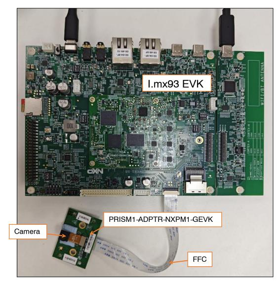
2. Below is an example to connect PRISM module to NXP i.mx93 and NVIDIA Jetson Nano.
