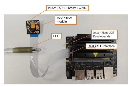
Figure 9. PRISM Module to NVIDIA Jetson Nano EVK
