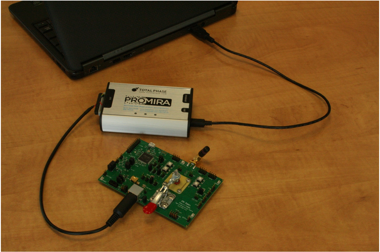
Figure 5. Connected Ezairo 7160 SL Hybrid Demonstrator Board, Windows PC, and Programming Box
