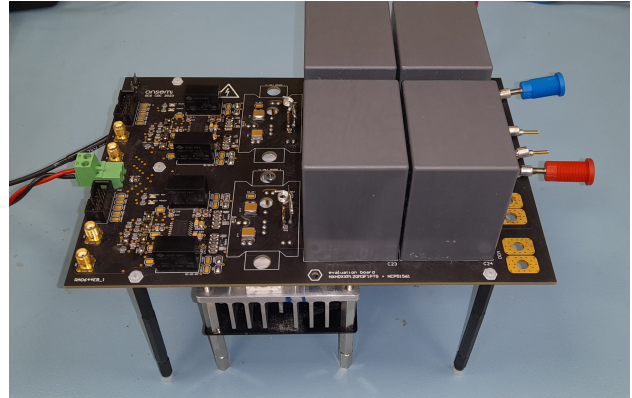
Figure 15. Application Board Placed on a Heatsink
