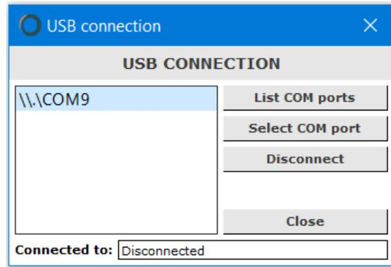
Click on the COM port in the list to choose the correct one and then click on the Select COM port button. The bottom should change the text to **Connected to:** COM port.
