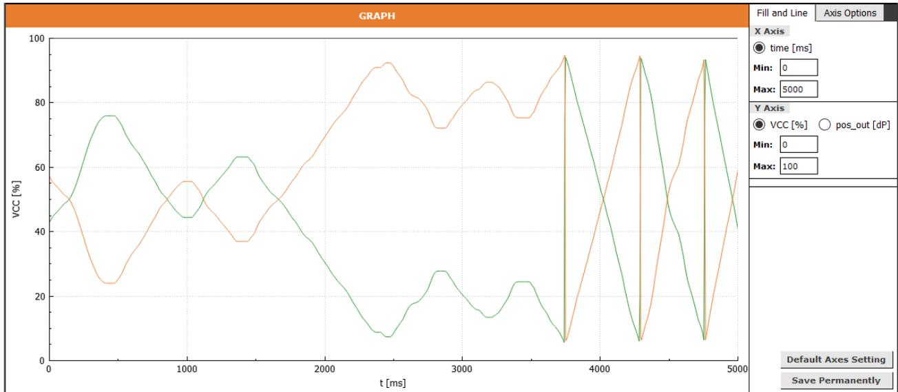
In the GRAPH part it is possible to see the data from chips which are read when AUTO READ button is pressed. On the right there is a panel for graphical settings. It is possible to set:
