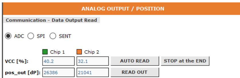
In “ANALOG OUTPUT / POSITION” it is possible to read the position data from two chips. First it is necessary to choose the communication interface for reading the data:
