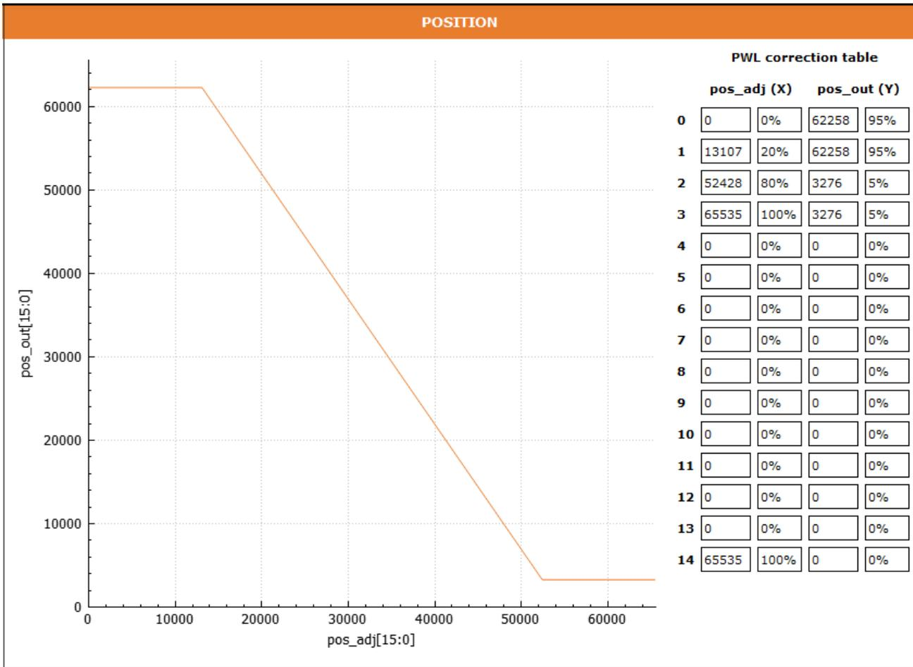
In this part it is possible to set the PWL correction table. On the left there is a graph which shows the programmed output curve. On the right it is possible to set pos\_adj and pos\_out in dP or in percentage.
