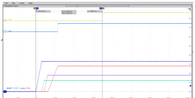
Figure 15. Power-up Sequence Example
